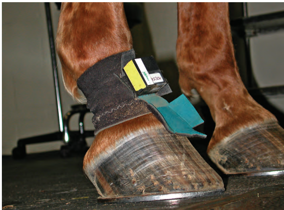
The Lameness Locator evaluates soundness based on the vertical motion of the torso, so the gyroscope placed on the horse's right foreleg should have no bearing on how the horse's torso accelerates and decelerates.
