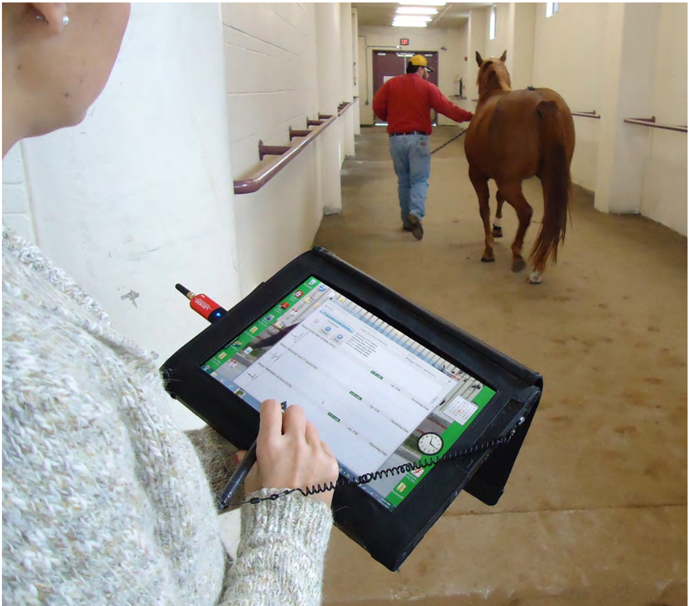
Bluetooth technology captures data from the Lameness Locator sensors and transfers the information to a wireless tablet with software that produces a computer readout with the data results.
